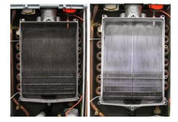
Heat exchanger effect (siloxanes 5 ppm D5)
