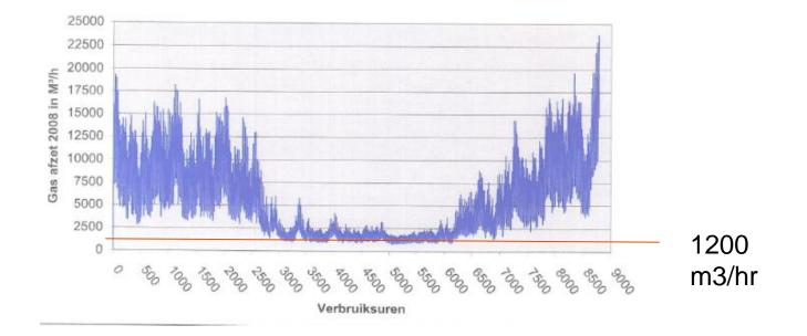
Feed in: for example Max 1200 M3/hr. (small City) Agricultural area's much lower. Average size plant ca. 300-400 m3/hr. Feed-in capacity is limited, often one or two per Gate Station grid
