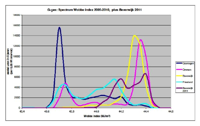
Quality change is a current ongoing process, installations can handle a specific bandwidth, with additional extra safety margins
